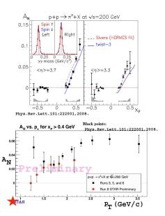
Figure 1: Top: Asymmetry  $A_N$  as measured in this experiment is shown as a function of Feynman  $X_F[1]$ . The dashed line is a fit to the Sivers model [2] and the solid curve is a fit two a twist 3 calculation[3]. Bottom: Asymmetry  $A_N$  as a function of  $p_T$  for  $X_F > 0.4$ . The data points shown as black squares was collected prior to 2008 (Run 8). The red circle data points are from new 2008 FPD data.
